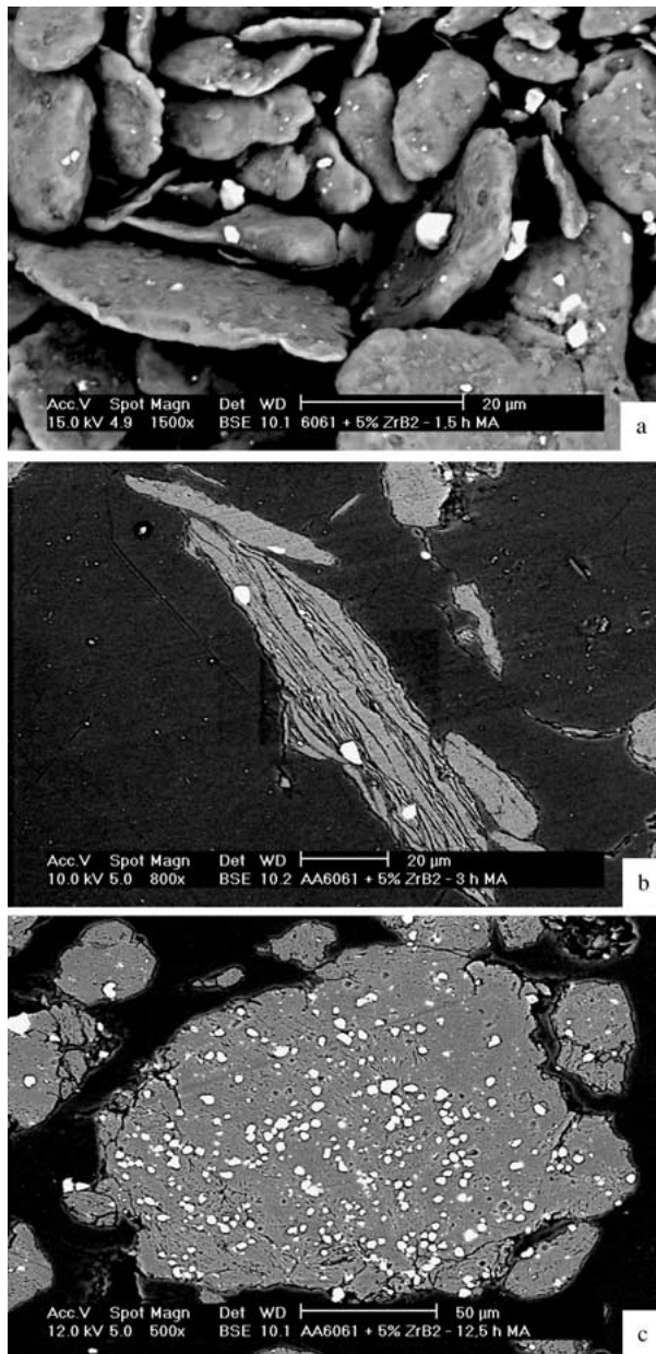
Figure 2 Evolution of powder morphology: (a) ZrB_2 reinforcement particles located on the flattened aluminium A6061 particle surfaces, observed after 1.5 h of mechanical alloying, (b) ZrB_2 reinforcement particles trapped on the interfacial welding boundaries of aluminium particles, observed after 3 h of mechanical alloying, and (c) composite particles of A6061 reinforced with 5% ZrB_2 obtained after 12.5 h of mechanical alloying.
